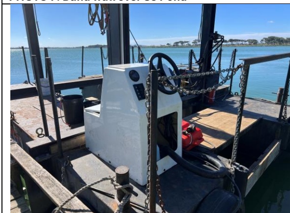
PHOTO 9: Refuelling boat – the holding area of the vessel is sealed and would contain any spills
