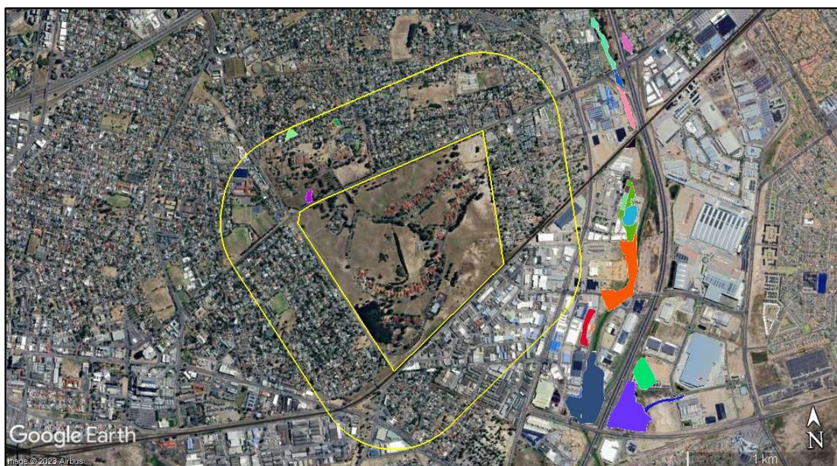
Figure 8: City of Cape Town Wetlands Layer (BioNet, updated 2018). The wetland features identified to the north west (indicated as green and purple polygons) of the site and within the regulated zone are upslope of the site (i.e. the proposed development poses no risk to these feature). The remaining features are beyond the regulated zone.
