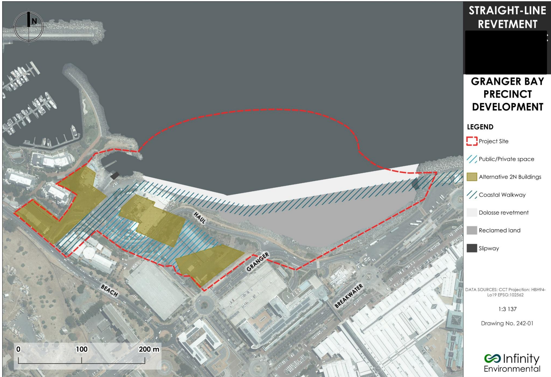
Figure 4—10: 2018 Scheme: Straight-line revetment with more limited public space and access to the water's edge
