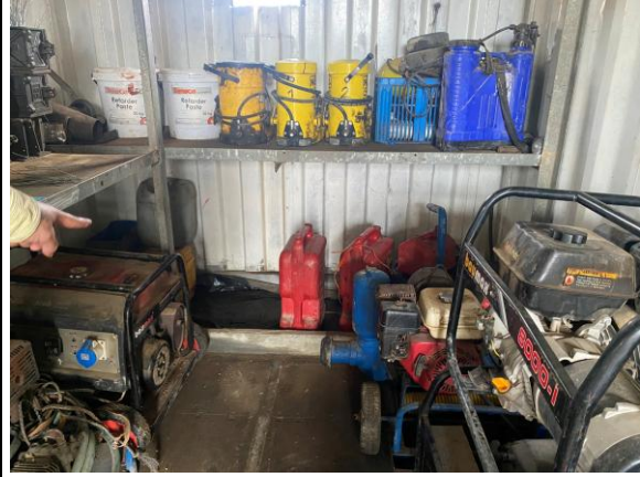
PHOTO 20: Secure petrochemicals storage in secure site container – with ventilation and spill trays
