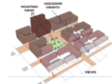
FIG 5 CASCADING BUILDING HEIGHTS TO OPTIMISE VIEWS OF THE WATER AND OF TABLE MOUNTAIN FROM THE WATER. BUILDINGS TO BE OF AN APPROPRIATE SCALE TO THE WIDTH OF THE STREETS ONTO WHICH THEY EDGE
