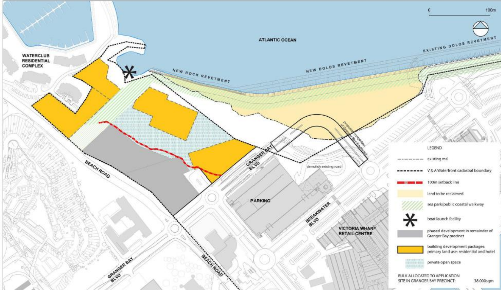
Figure 44: 2019 approved Dolos revetment with land reclamation
