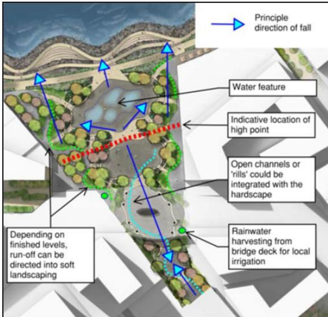
Figure 2-27. Proposed Granger Walk park with relevant stormwater management features
