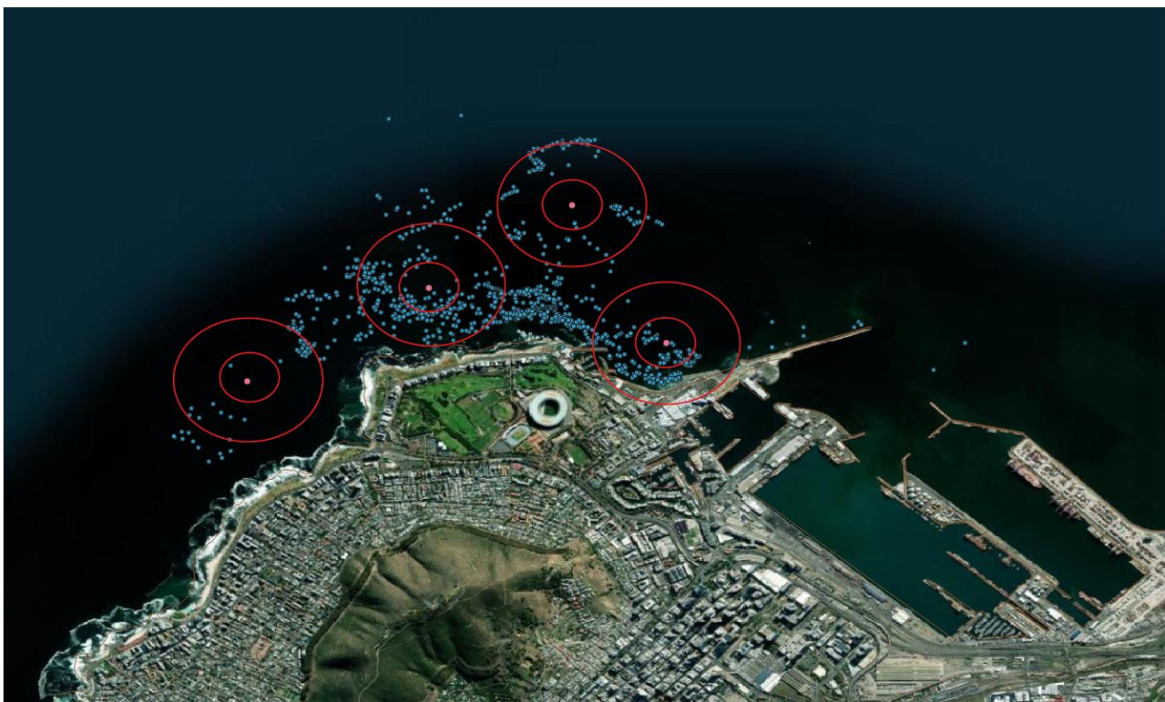
Figure 8-1: Suggested deployment plan for long-term acoustic monitoring of dolphins and whales in Granger Bay and Three Anchor Bay area (Blue-dots: Known locations of Heaviside's dolphins, Red dots: proposed location of hydrophones and Red circles: 200m effective detection radius and 500m maximum detection radius for Heaviside dolphins.
