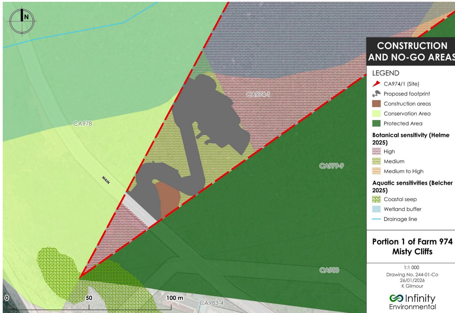
Figure 2: All areas except the proposed footprint and construction areas are no-go areas
