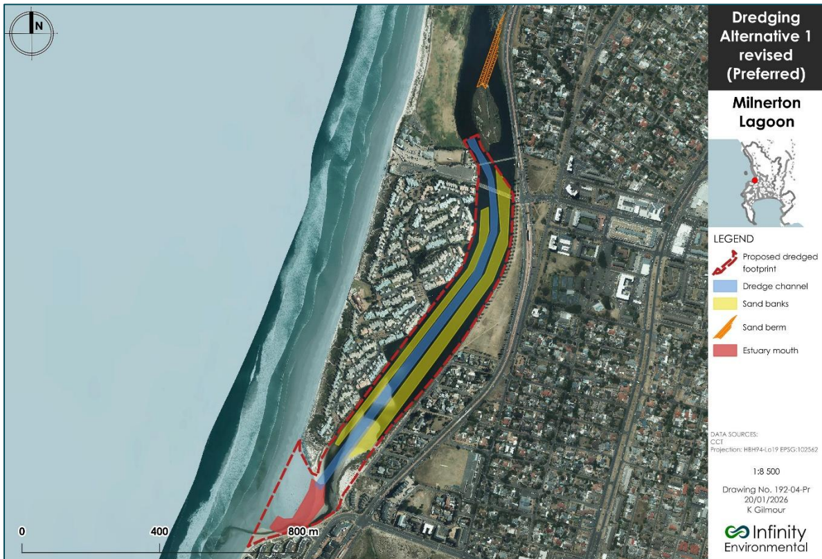
Figure 2: Schematic of the updated preferred alternative, illustrating the proposed dredging area (blue) in the Milnerton Lagoon, with the excavated material (yellow polygons) placed on either side of the channel. The proposed sand berm is highlighted in orange, while the dotted outline depicts the precise footprint of the dredged area. The design has been amended slightly since the draft BAR based on comments received, to maintain deeper water along the western bank immediately downstream of the Loxton Road bridge.
