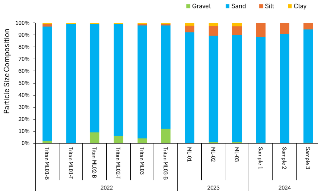
Figure 3-17. Mean cumulative percentage contribution of sediment particle grain size fractions (gravel, sand, silt and clay) sampled at sites (see Figure 3-15) on the lower Diep Estuary in December 2022, November 2023 and September 2024 (data courtesy of Gus Hojem and Jeremy Rose, 2024).
