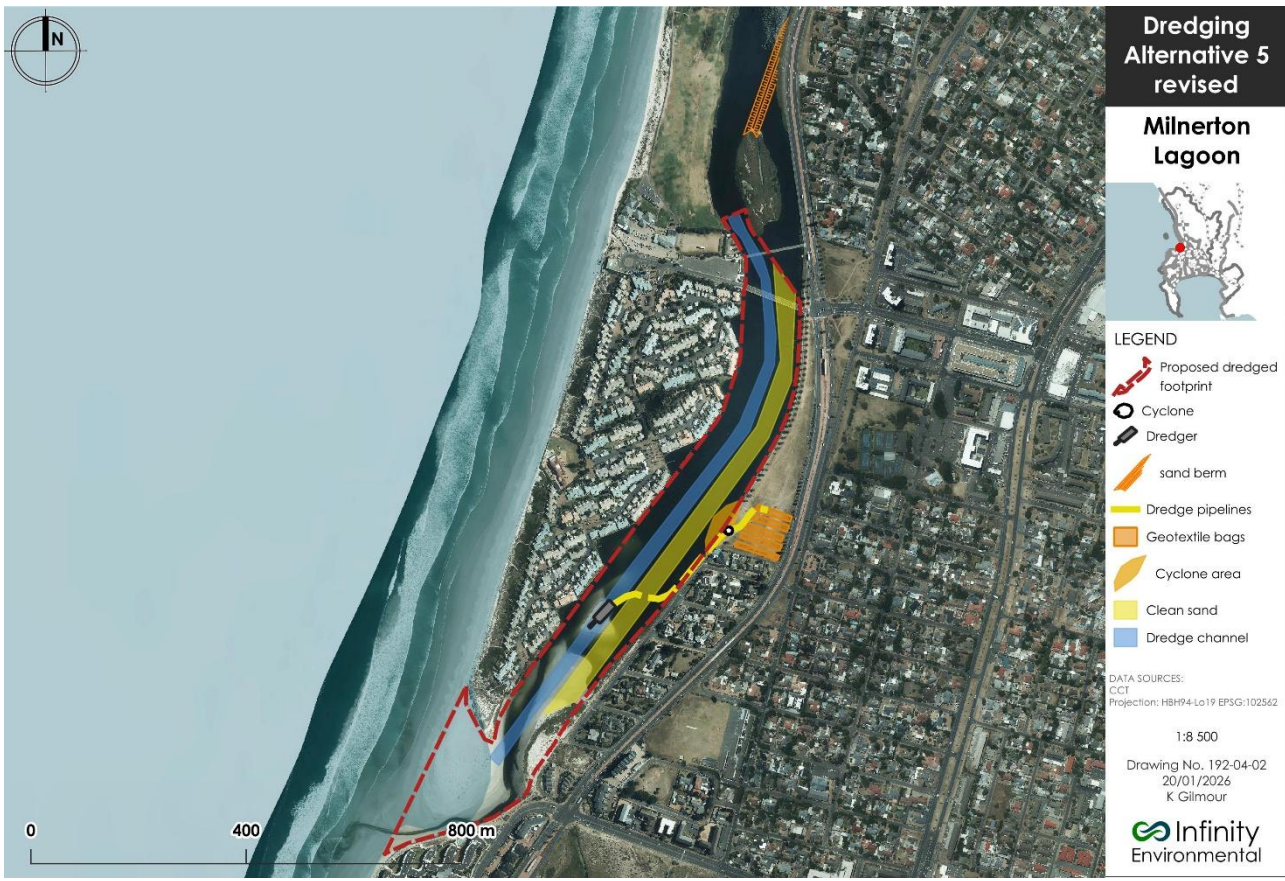
Figure 3: This schematic presents the design and layout Alternative 5 – the proposed dredging with off-site disposal.
