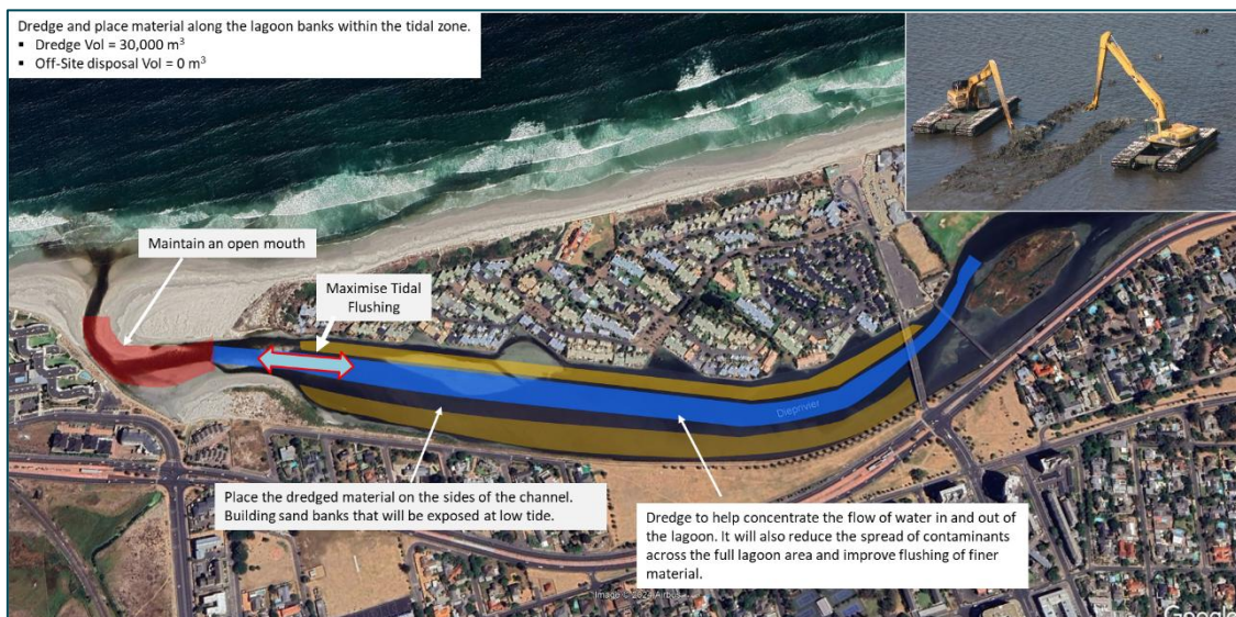
Figure 2: Dredging option 1 schematic – dredging proposal without deposition of material offshore or within the estuary mouth.
