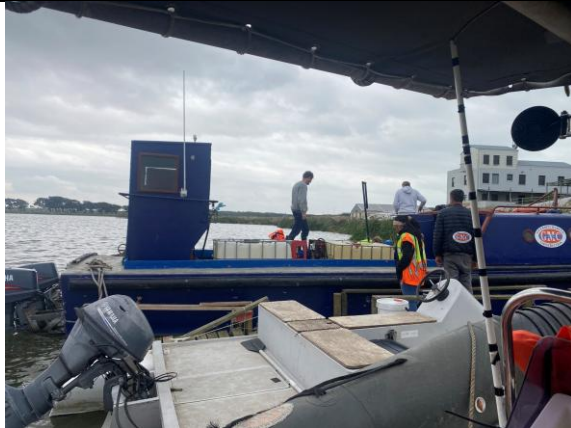
PHOTO 11: Refuelling boat with flow bins – the holding area of the vessel is sealed and would contain any spills
